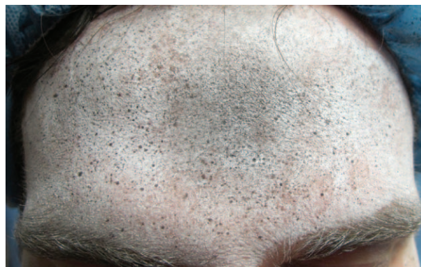
Fig. 1. A subject prepared for imaging. White foundation and black speckle makeup are applied to each patient. The speckles are tracked by the digital camera, and their displacement is quantified with ARAMIS.
